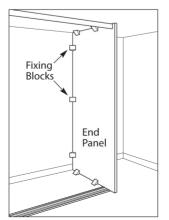
End Panels which can be sourced from most DIY stores. Scribe to fit against the desired wall and attach using Fixing Blocks.
