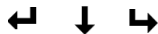
3-port valve Only the flow direction or current switching position is indicated.
