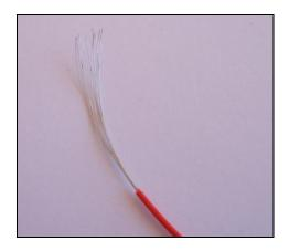
2. Twist the wire between your finger and thumb to stop fraying
