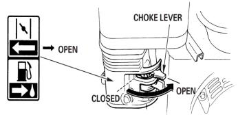
5. If the CHOKE LEVER was moved to the CLOSED position to start the engine, gradually move it to the OPEN position as the engine warms up.
