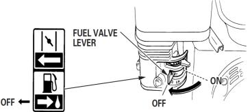
3. Turn the FUEL VALVE LEVER to the OFF position.
