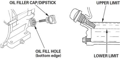
5. At the correct full level the oil will sit on the edge of the threads on the engine oil filler neck.
