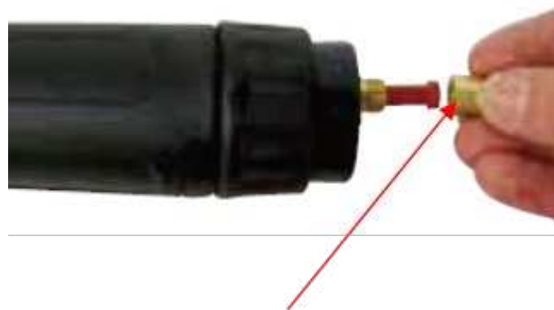
(2) Remove the liner retaining nut.
