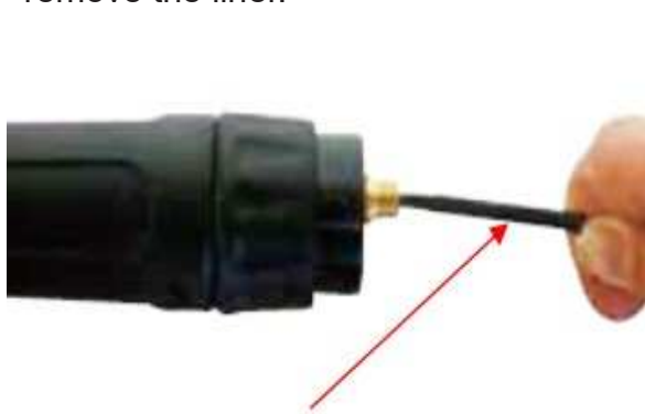
(5) Carefully feed in the new liner in short forward and movements down the torch lead all the way to exit the torch neck. Be care-full not to kink the liner.
