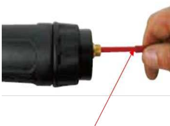
(3) Carefully pull out and completely remove the liner.
