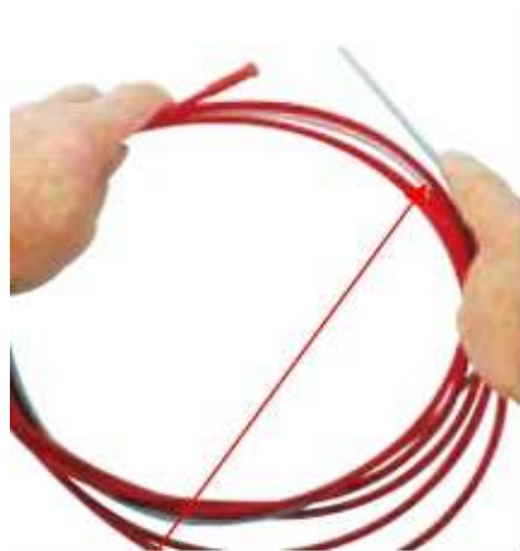
(4) Carefully unravel the new liner.
