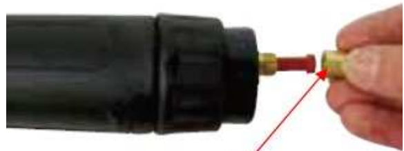
(2) Remove the liner retaining nut.
