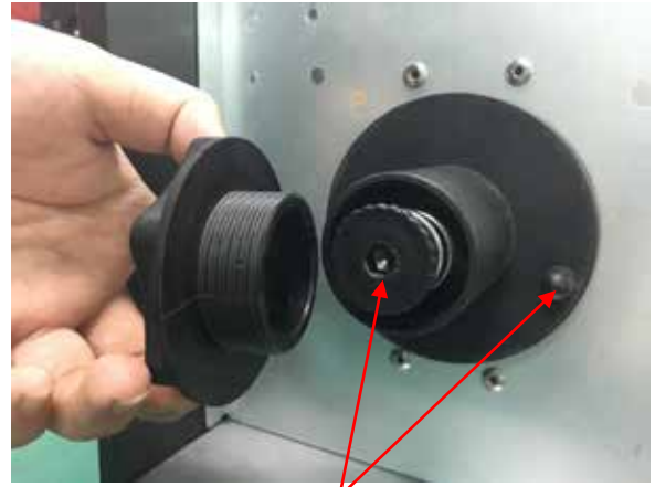
(2) Note the tension spring adjuster and spool locating pin.
