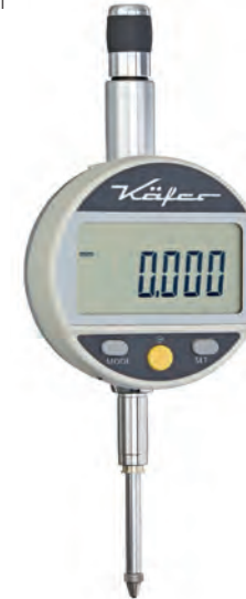
Digital Dial Gauge MD 12 TOP Reading: 0.01 mm / 0.0005" Range: 12.5 mm / .5" Bezel Ø: 60 mm Output: RS 232 / DIGIMATIC / USB Maximum Error: 20 µm £171.30
