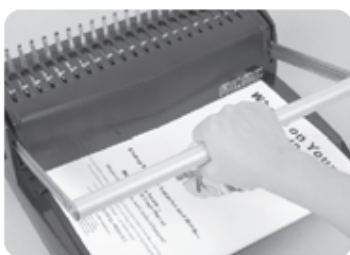
(Fig. 4) Pull the Handle all the way down until it stops to punch completely through paper
