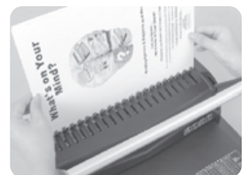
(Fig. 6) Load punched sheets directly onto the opened comb
