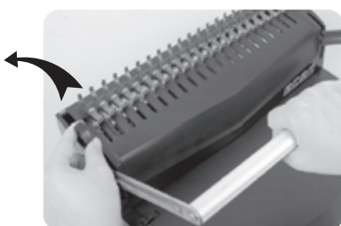
(Fig. 7) When finished, release the Comb opening lock and return the Handle to the original position
