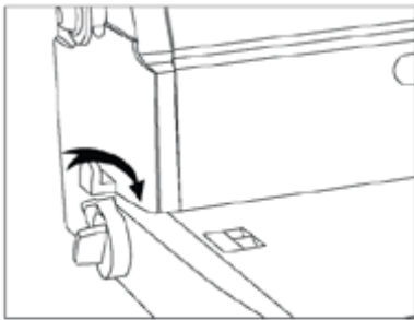
(Fig.7) Extra large punching guide: Rotate the Extra large punching guide and expose the desired registration pin for punching.
