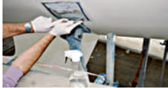
Wet scrape to remove old antifouling
