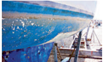
Paint blisters and lifts
