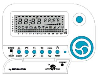
becomes the master of the entire system, therefore almost all the functionalities, as the setting of heating and hot sanitary water set-point or the control of system status, are directly executable by it, in relation with the kind of application on which the board is used. By means of the remote control it is possible to restore (**RESET**) the system from the non-volatile lock status.
