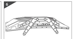
Line the base plate to the stand holes and tighten all 3 screws up, one by one
