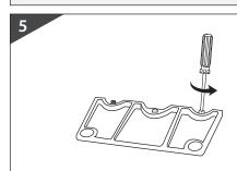
Start off by removing the 3 screws on the base plate with the screwdriver provided
