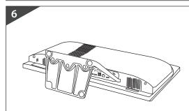
Line the base plate to the stand holes and tighten all 3 screws up, one by one
