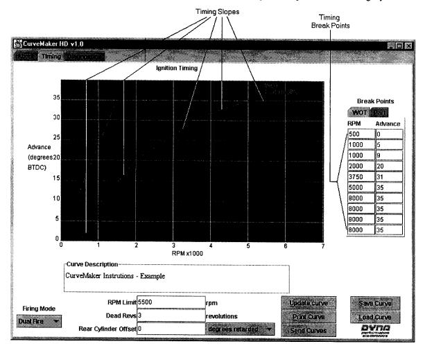
Each ignition curve is defined by timing slopes. A timing slope connects each Break Point with the next. There is not a timing slope between two points if the ignition timing is a vertical line. In the above example, the only line on the Timing map that is not a timing slope is the vertical line at 1000 rpm that goes from 5 to 9 degrees of advance. The ignition accepts a maximum of 8 timing slopes per timing curve.
