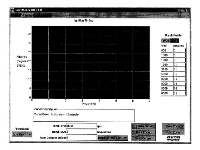
Select the "WOT" Tab to adjust the Wide Open Throttle curve. Move the mouse over the Advance value next to 2000 RPM, and click the mouse button to edit the value. Enter the new value for the Advance. Move the mouse over the rpm value, click and enter 1950 rpm.
