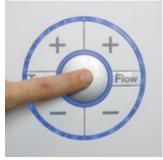
+ To **start** push the larger circular central button which has an illuminated light around it to activate the unit
