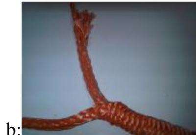
Step 8: Smooth the rope down starting at the thimble end so that the tail disappears back inside the rope.
