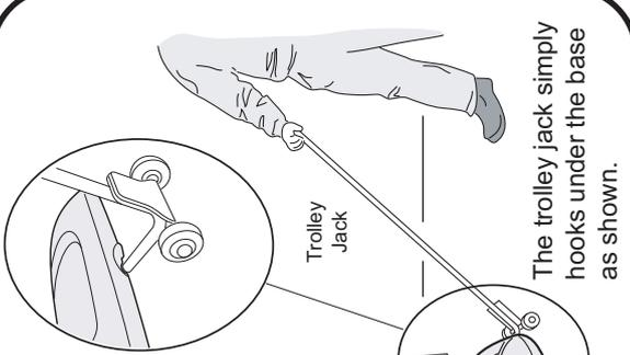
The trolley jack simply hooks under the base as shown.
