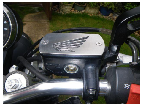
Image showing correct placement of cover. Note retention of original cover underneath
