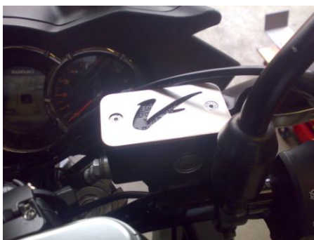
Image showing correct placement of cover. Note retention of original cover underneath
