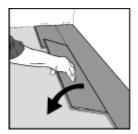
8. Place the board tight to the short end of the previous board and fold down in a single action movement ensuring the short joint "clicks" and locks correctly. <u>Do not force the end to locate using excessive pressure</u> or a hammer as the end section of the profiles may be damaged.
