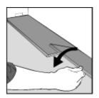
3. Fold the board down with a single action movement to locate the header joint **ensuring** the joint "clicks" and locks. <u>Do not force the end to locate using excessive pressure</u> or a hammer as the end section of the profiles may be damaged.
