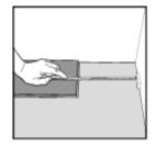
4. At the end of the first row, place a 6mm expansion gap spacer against the right hand wall or skirting board, and measure the length of the last board to fit.
