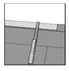
10. Measure the width of the final row of boards. The minimum 6mm expansion gap must again be left at the edge
