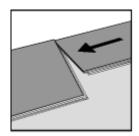
2. Second board, first row. Locate the board end into the short end of the first one ensuring the front and back edge line up accurately.
