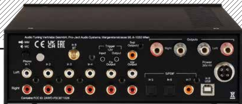
ABOVE: MM/MC phono and three line ins, plus a sub, fixed and variable pre outs are offered on RCAs alongside USB-B (192kHz/24-bit; DSD256), BT antenna and coaxial plus two optical S/PDIF (192kHz/24-bit) digital ins. Power connects via a 4-pin DIN while speaker outs are on insulated 4mm sockets (now better placed than before)
