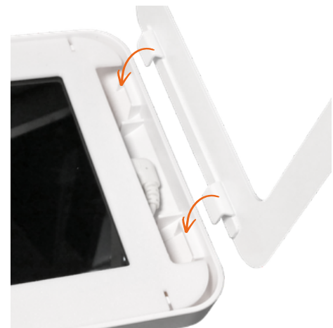
Metal hooks slot into place
