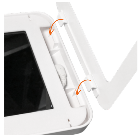
Metal hooks slot into place
