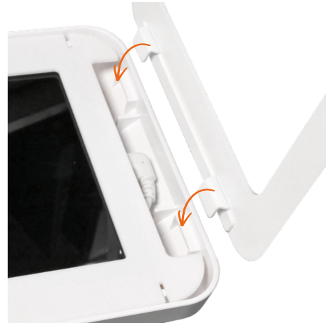
Metal hooks slot into place
