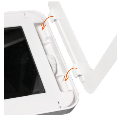
Metal hooks slot into place
