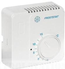
A thermostat designed for connection to our general-purpose transmitter or GSM dialler to provide instant warning of a critical temperature in a greenhouse / poultry shed etc. Will monitor for under-temperature or over-temperature. Set-points between -5 and +35 degrees.
