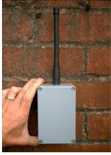
A FarmGuard transmitter with built-in batteries. Transmitting range to the receiver is about 400—500m. This can be extended using a whip or yagi antenna. It can be triggered by a relay contact (normally-open or normally-closed), a float switch, a mains-failure module, a thermostat or any other switching mechanism.
