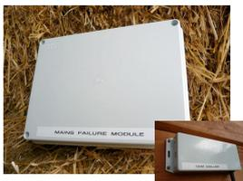
A single-phase mains failure module. It simply plugs into a 13A socket and triggers the instant the power goes off. It features a battery backup and a GSM dialler to raise the alarm when a critical power failure occurs and report the condition to your mobile phone by text message or voice call. It will report to up to ten phone numbers (landline and mobile) and comes supplied with a SIM card and a linked swipe-card for easy topping up.
