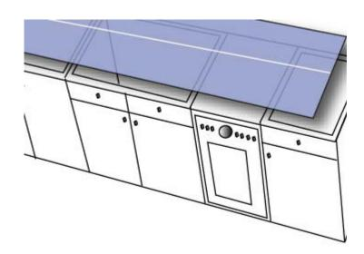
NOTE: If seams are placed on structures without full support, the top may crack and seams may have to be replaced
