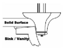
Tips: • In order to visualize the sink and determine how it will bond to the surface, it may be helpful to pre-cut the sink cutout or make a pilot hole in the centre.
