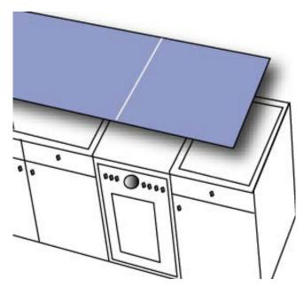
Try to avoid placing the seam over the dishwasher. However, if there is no alternative, the seam must be reinforced. If it is impossible to avoid dishwasher, make sure to note it on the template.
