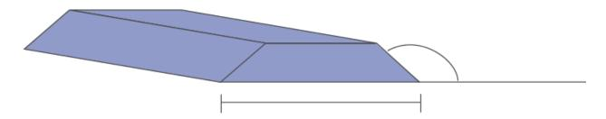
Note: All side edges need to be cut to a 45° angle to prevent any stress.
