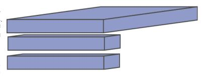
Note: There must to be a width of at least 25mm (1") in order to use this method. 50mm (2") is recommended for the buildups.
