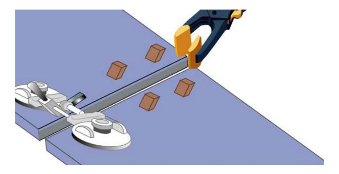
Make sure you research and become familiar with the various clamping methods before you apply it to the seaming process. If you choose the wood block method, you will have to apply hot glue along the seams before applying the adhesives.
