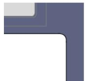
The seams need to be at least 25mm (1") from the end of the radius of any inside corner.
