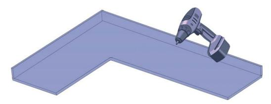
Note: Twisting or forcing the drill while drilling the hole can create cracks in the countertop.
