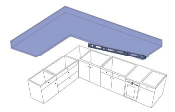
After setting all the pieces in place, dry fit the entire top. If you see any discrepancies, make the corrections at this time before you start the installation process. Check the following:
