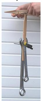
The weight of the strut & spanners on the scales 1.484 KG (not bad for a little magnet).
