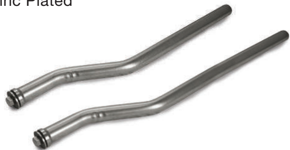
Wingstay Single Bolt Fitting Direct to Chassis Zinc Plated
